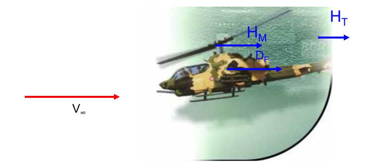
Total Drag= Fuselage Drag ( $D_F$ ) + H-force on main rotor ( $H_M$ ) + H-force on the tail rotor ( $H_T$ )
