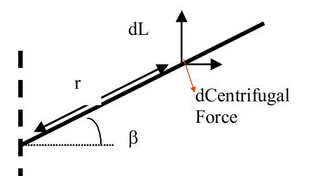
We assume that the rotor is hinged at the root, for simplicity. This assumption is adequate for most aerodynamic calculations. Effects of hinge offset are discussed in many classical texts.
