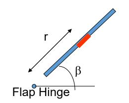
Small segment of mass dm With acceleration  $r\ddot{\beta}$
